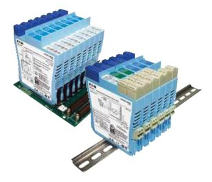
The MTL5500 clips quickly onto DIN rail, so it is compatible with the industry-standard mounting system. Wiring is simplified by plug-in safe- and hazardous-area connectors, and a power plug which accepts a power bus; it all leads to quicker insertion, fewer wiring errors and trouble-free, tidier installations.
